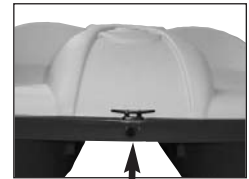
Photo #4 Drain Plug Location
